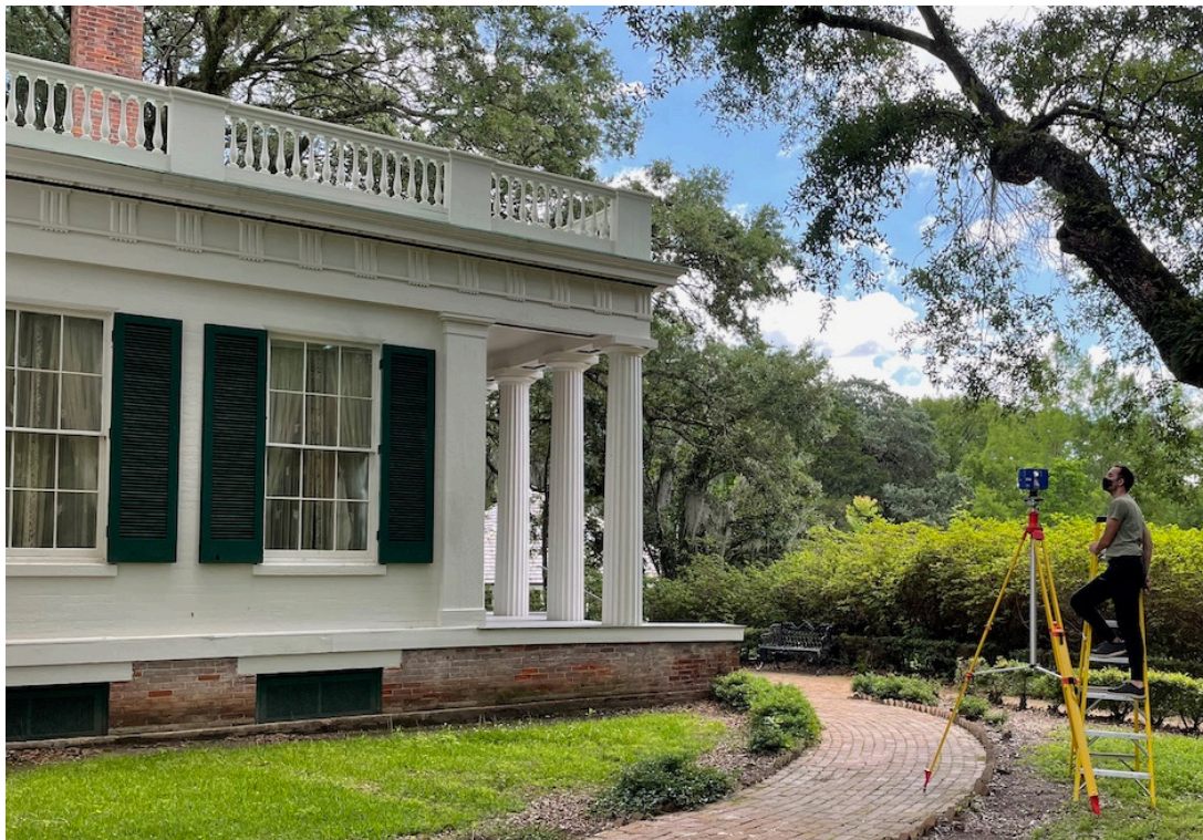
Figure 4: Scanning the façade using the Faro Focus 3D mounted to a Seco giant elevating tripod. Normally drone photogrammetry would be used to document higher portions of an exterior façade, however large oak trees in close proximity prevented the use of drone in this instance.
