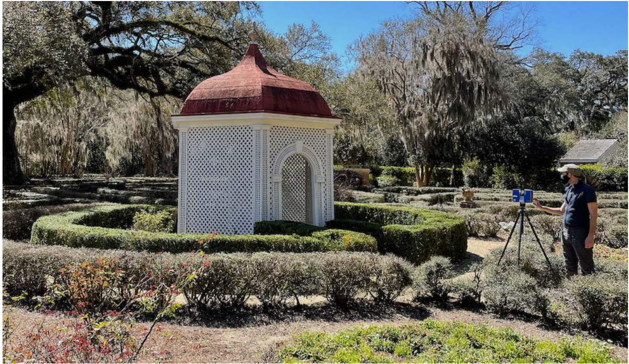
Figure 3: The team used a Faro Focus 3D to collect point cloud data. Here Brendan Harmon is scanning the outside of an original summerhouses in the south formal garden. Image from site visit on March 7 th , 2021.
