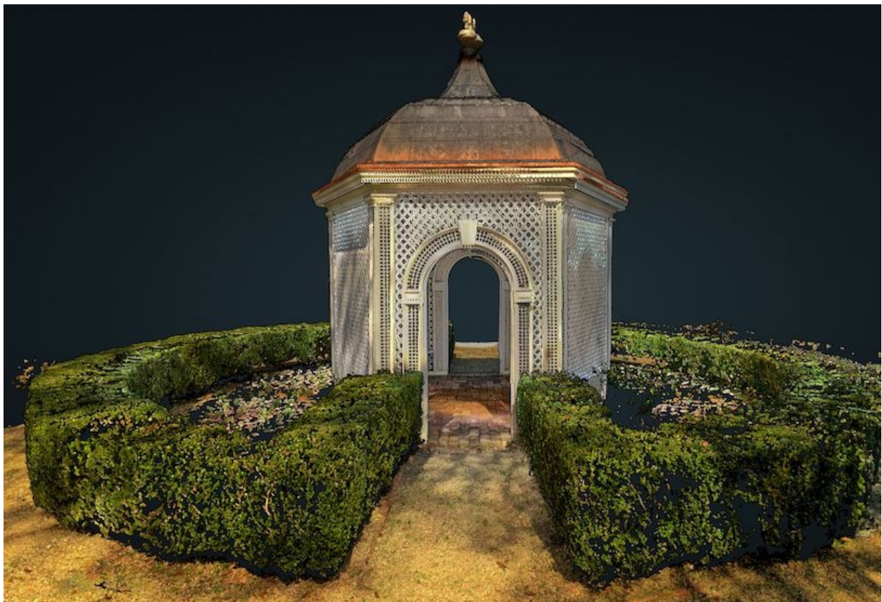
Figure 16: A point-cloud model of the summerhouse in the south formal garden was created
