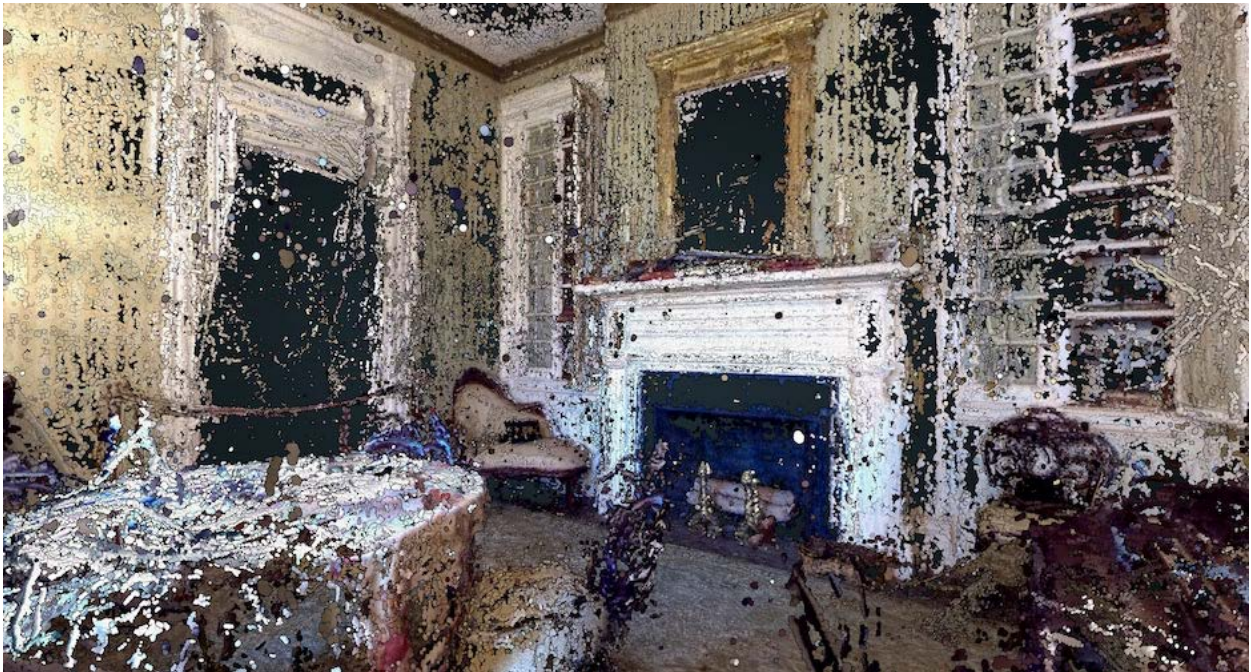
Figure 21: Screenshot of point-cloud generated from 360° camera photogrammetry. This proved unsuccessful because there was too much noise.
