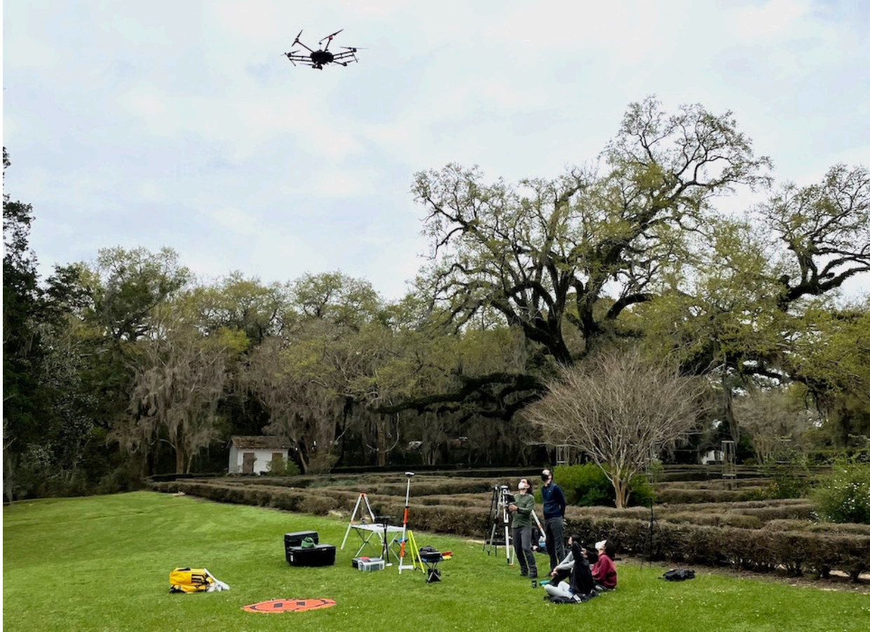
Figure 2: The research team used a DJI Matrice 600 Pro hexacopter to collect imagery for photogrammetry. Several missions were flown over four separate site visits. Image from site visit on March 20 th , 2021.
